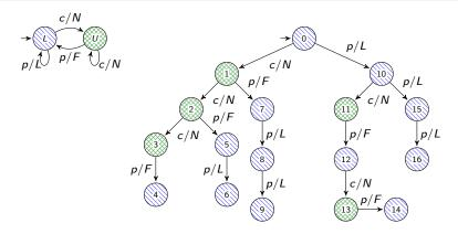
Test suite  $T = \{cccp, ccpp, cppp, pcpcp, ppp\}$ , represented here as a tree, was generated using SPYH-method and is  $\mathcal{U}_3$ -complete for machine on the left. Test suite is not  $\mathcal{U}_1^{\{\epsilon,c\}}$ -complete.
