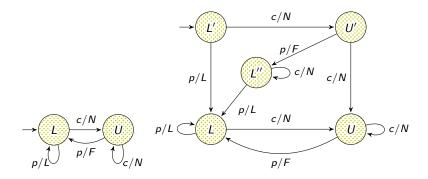
Mealy machine on the right is contained in fault domain  $\mathcal{U}_1^A$ , for  $A = \{\epsilon, c\}$ , since all states can be reached via at most one transition from states L' and U' that are reachable via A.
