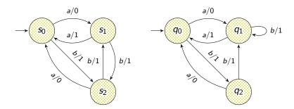
Test suite  $T = \{aaaa, abaa, baaa, bbaa\}$  for specification S on the left is  $U_3$ -complete. SUT M on the right does not pass test abaa.
